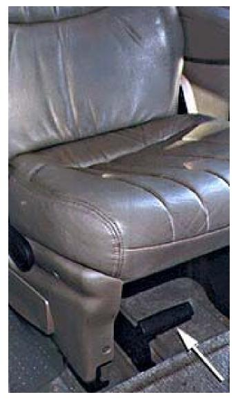
Seat is designed to be removed. To someone who is unfamiliar with this seat would think the handle under the seat is to adjust it but it is actually to remove the seat for more storage. The Handle is improperly labeled. I would fix this problem by moving the handle under the seat and labeling the handle clearly
